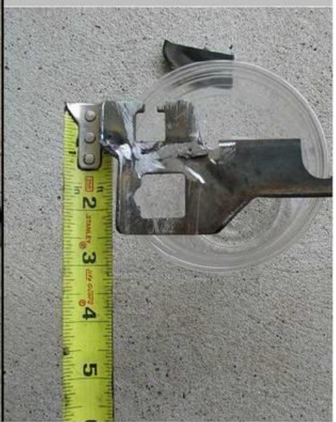
Bracket Welded Together
